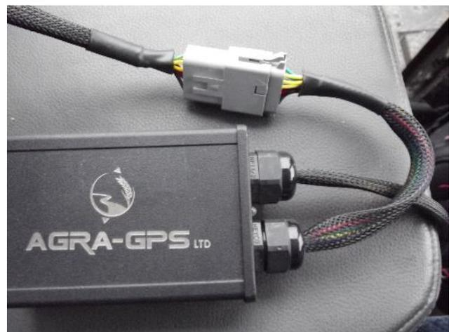
To install the machine to monitor adapter, remove the first 31-Pin circular Deutsch cap from its connector located on the left side of the cab. This will be the one located closest to the front of the machine.
