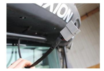
Now drill a hole fort he cable which goes tot he display. Run the cable out of the cover. Then reassemble the covers again.
