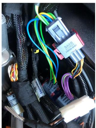
Now connect the grey 6Pin Deutsch connector of the adapter.
