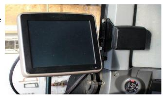
Another option is using two RAM mount 1.5" ball (RAM-202U) and a 4" double socket arm (RAM-201U).
