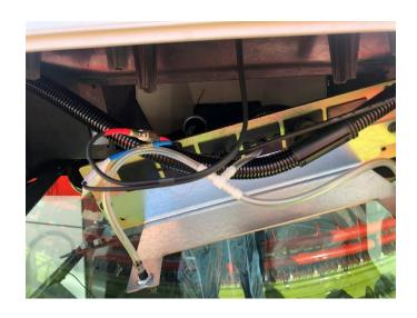
After the cable is out of the roof and the plastic covers are mounted again reassemble the 12-pin deutsch connector.
