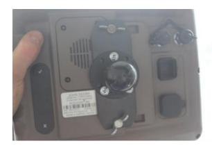
The picture shows a JD 2630 display mounted using a RAM mount hardware and the standard Claas Lexion "rail".
