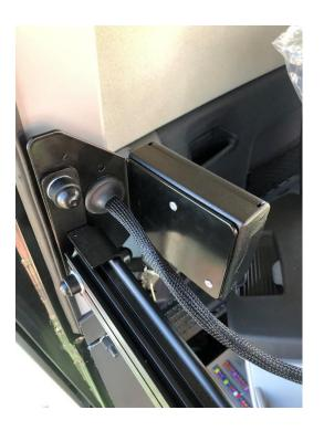
Once all cables are connected you may power up the system by simply turning the ignition key. The Claas-JD Bridge should show a blinking green LED after a few seconds and your JD display should be booting up.
