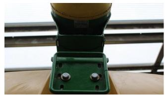
Optional base plate for Claas Lexion roofs. It is mounted onto existing screws in the roof and does not require drilling into the roof!
