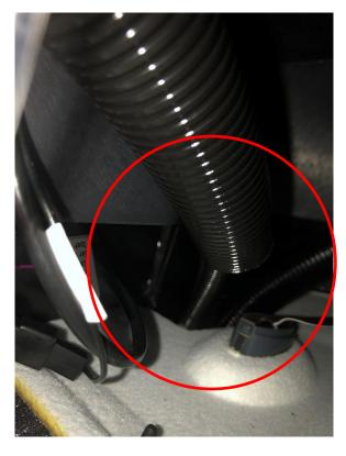
Remove the wedge in the 12-pin deutsch connector and carefully pull the cables backwards out of the connector. You will need a small flat screw driver to release the plastic clamps inside the connector. MAKE A NOTE OF THE PIN/CABLE LAYOUT BEFORE YOU REMOVE THE CABLES! Disconnecting the deutsch connector allows you to run the cable behind the plastic and through the cable canal. May put some isolation tape around it to protect the pins!
