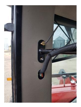
Now remove the door latch which still holds the plastic cover in its place.
