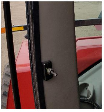
Find the connector labelled C602 behind the panel. Open it and insert the provided AgraGPS harness.
