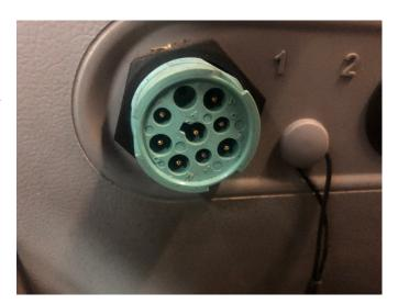
Locate the InCab ISO BUS socket of the tractor.
