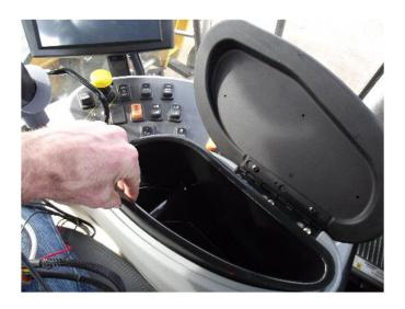
Disconnect the 3-pin Deutsch connector from its terminating plug inside the armrest. Insert the 3-pin Deutsch plug of the AgraGPS adapter harness to the connector.
