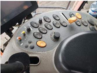
The autosteer is engaged with the "Resume" button in the control handle.
