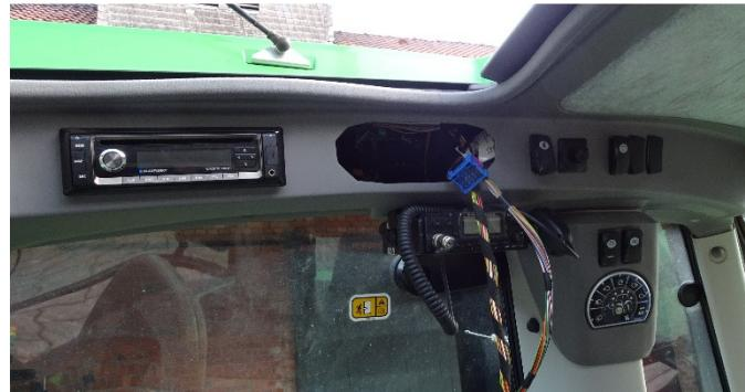
Find the blue 15-pin connector XC10 and open the connection. The connector is located to the right of the opening. Insert the Agra-GPS adapter harness into the 2 \* 15-pin connection points and place the Deutz-JD Bridge in the opening to the right.
