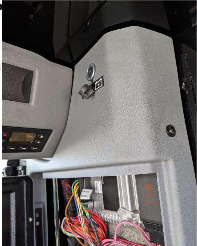
Use the two diagnostic port connections to connect to the MasseyCombine JD-Bridge. The main diagnostic port of the MasseyCombine-JD Bridge (labeled Main) is connected to EDT#2 'AUTO', while the secondary diagnostic port of the MasseyCombine-JD Bridge (labeled Secondary, and contains only 1 green and 1 yellow wire) is connected to EDT#1 diagnostic.
