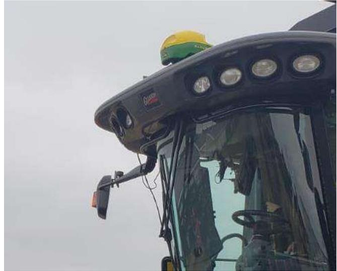
Use the provided adapter cable to connect the 12-pin deutsch of the JD GPS receiver with the 12-pin deutsch of the MasseyCombine-JD cable.
